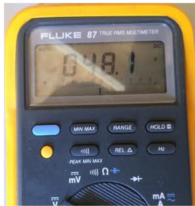
Figure 5-5: Output Voltage Reading of the MISO (PV Source ON)
