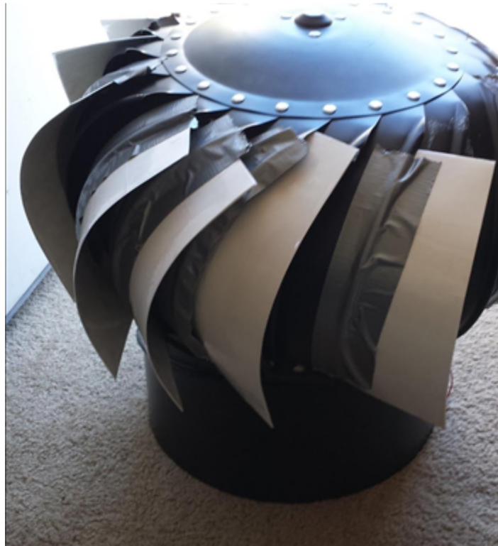
Figure 4-3: Additional fin extensions attached to turbine blades
