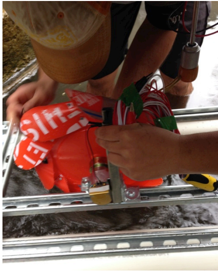
FIGURE 5-5: ORANGE TURBINE TESTING WITH FLOAT IN SLO CREEK
