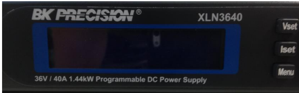
Figure 3: Programmable DC Supply for charging
