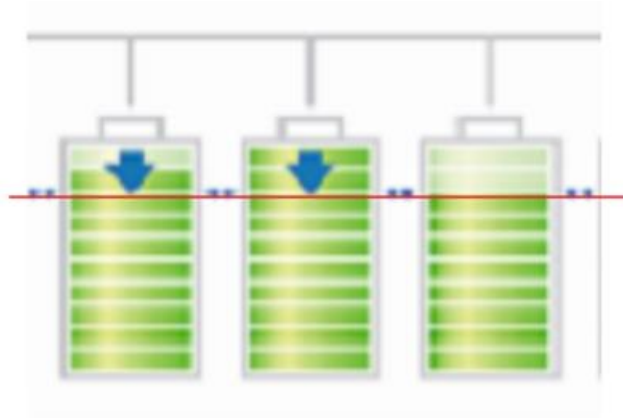
Figure 27: Cells dissipate to lowest SOC for passive cell balancing
