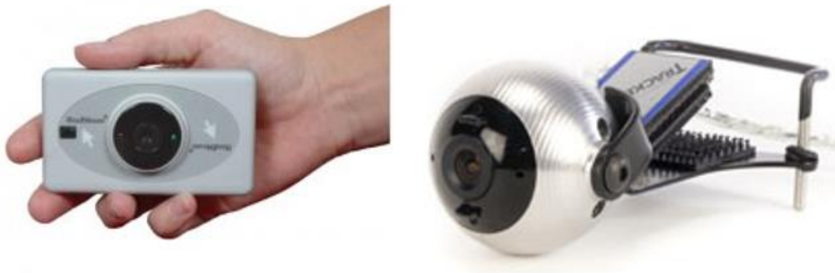
FIGURE 3: HEADMOUSE EXTREME (LEFT) AND TRACKERPRO (RIGHT), SCREEN-MOUNTED-CAMERA-BASED DOT-TRACKING SYSTEMS.
