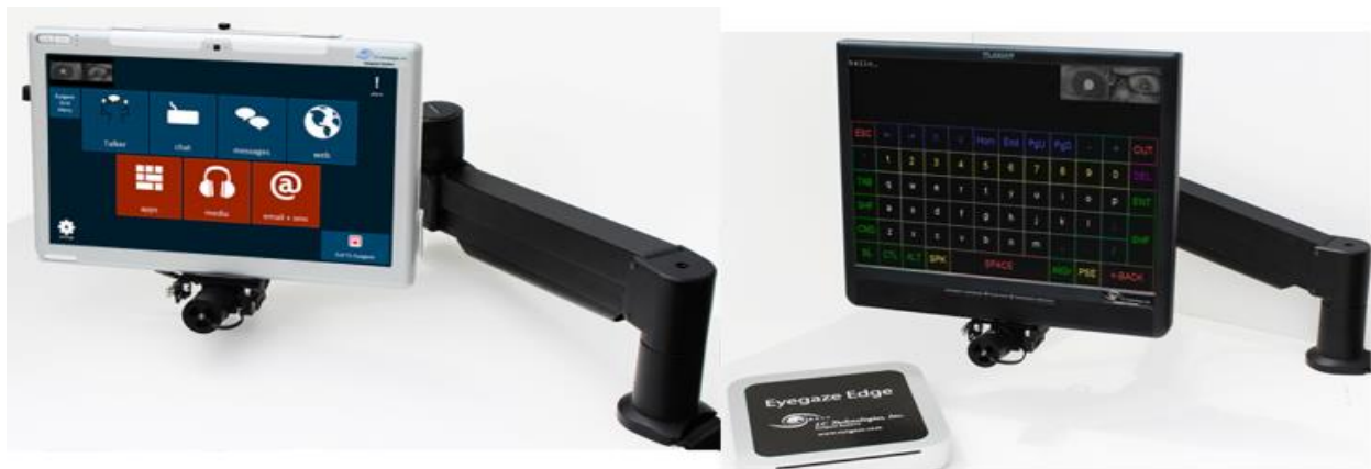
FIGURE 6: EYEGAZE EDGE TABLET AND EYEGAZE EDGE DESKTOP SYSTEMS WITH INTEGRATED EYE TRACKING HARDWARE
