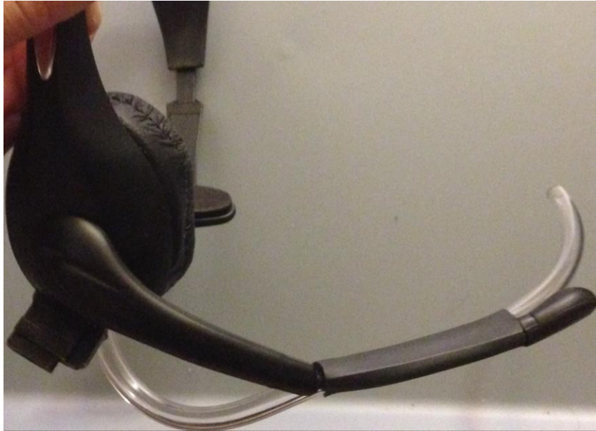
FIGURE20. COMPLETED HEADSET WITH RJ-25 JACK (BOTTOM LEFT) AND VINYL SIP-PUFF TUBING BEING ROUTED ALONG MICROPHONE BOOM USING HEAT SHRINK TUBING (BOTTOM).
