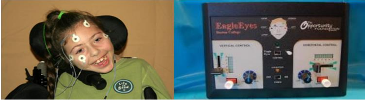
FIGURE 7: EAGLEEYES MYOELECTRODE SETUP (LEFT) AND CONTROL INTERFACE (RIGHT)
