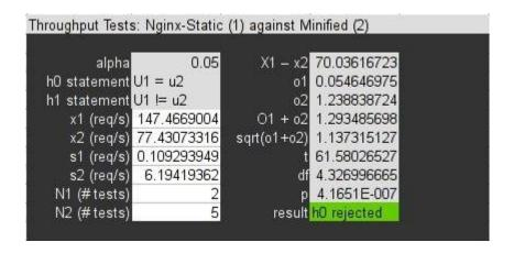
Load Tests, average mean of initial response time against the average mean of minified response time.
