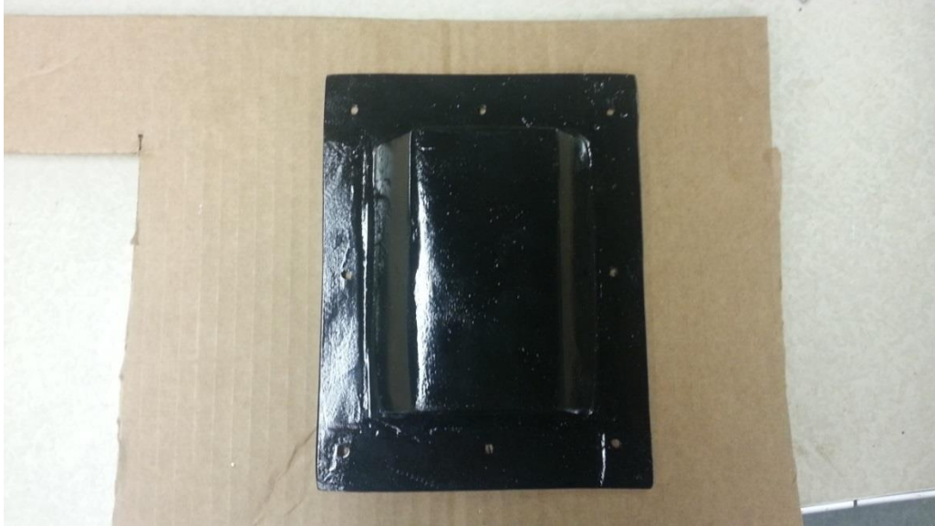
Figure 29: Contactor Plate sanded down and spray painted black.
