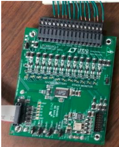
Figure 20: LTC6803-3 Demo Board (DC1653A)
