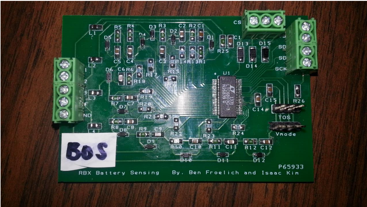
Figure 21: Battery Sensing Circuit with all components, output terminal blocks and jumper leads to set mode.
