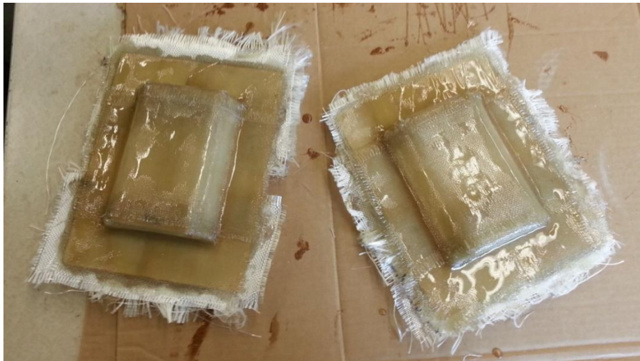
Figure 28: Contactor Plate made with Fiberglass cloth
