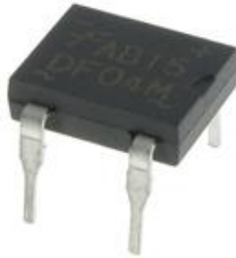
Figure 4-8: DF04M-ND Full-Wave Bridge Rectifier
