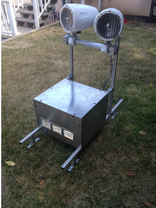
Figure 17. Different view of the Mobile Lark Scarer. The back of the MLS is also shown. The red handle of the ON/OFF switch can be seen as well as the cover for the male end of the charger receptacle.
