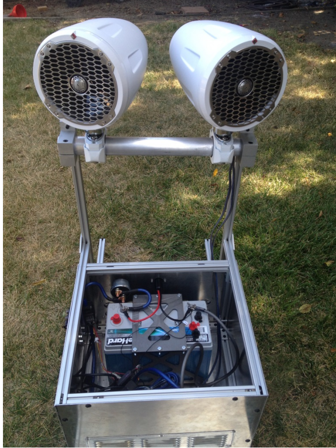
Figure 23. View of the MLS with speaker wire running from the amplifier shown.
