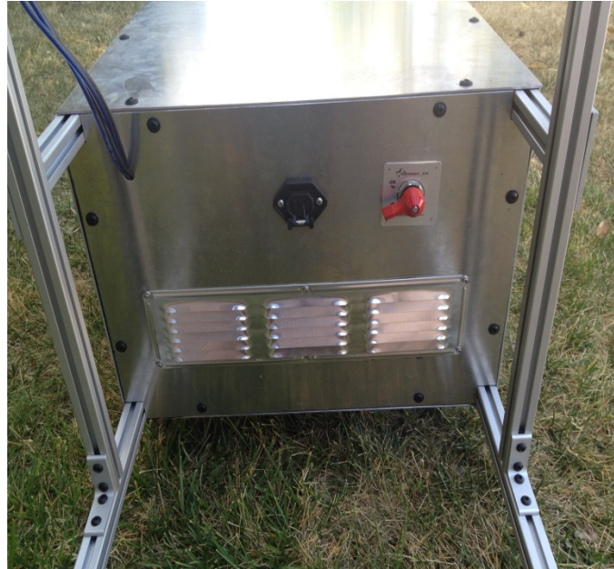
Figure 17. Different view of the Mobile Lark Scarer. The back of the MLS is also shown. The red handle of the ON/OFF switch can be seen as well as the cover for the male end of the charger receptacle.
