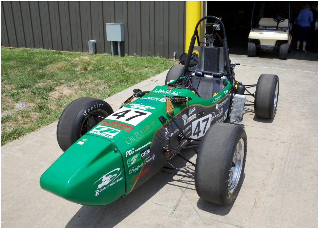
Figure 9.1 - Completed chassis with subsystems installed.
