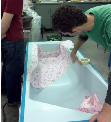
Figure 9.11 - Using fabric store remnants to make patterns for cutting the carbon.
