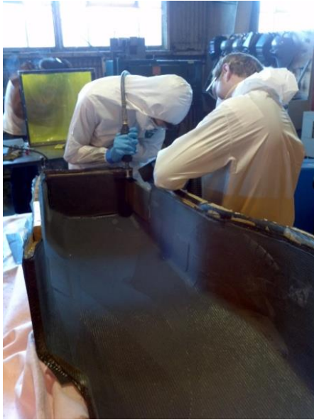
Figure 9.29 - Rough cutting the parts to prepare to bond the two halves together.
