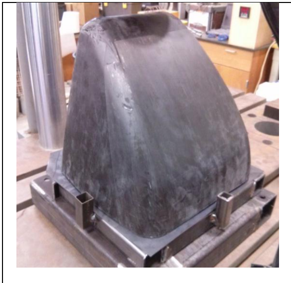
Figure 3: Attenuator as Constructed
