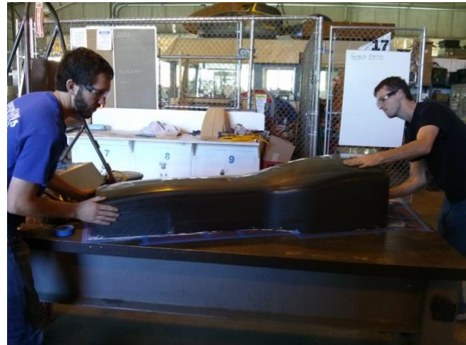
Figure 9.30 - Sanding the mating surfaces flat using a frame table.
