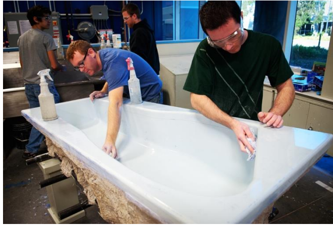
Figure 9.7 - The finished mold undergoing a final cleaning before the release agent is applied.
