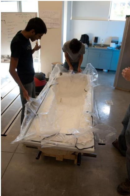
Figure 9.17 - The part under vacuum for one of the many debulking periods.
