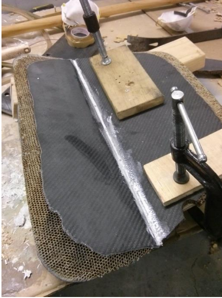
Figure 9.76 - Electronics cover undergoing cut and fold bend.
