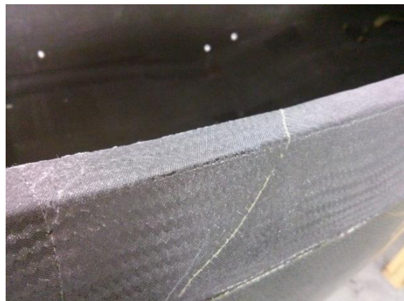
Figure 9.37 - The finished cockpit opening closeouts.
