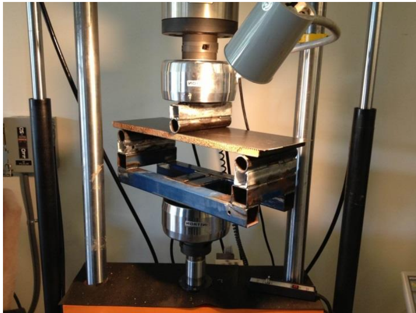
Figure 8.5 – Test setup picture for SAE three point bend test in accordance to rule T3.31. The rig had a span of 20 inches and could accommodate a specimen up to 8 inches in width.
