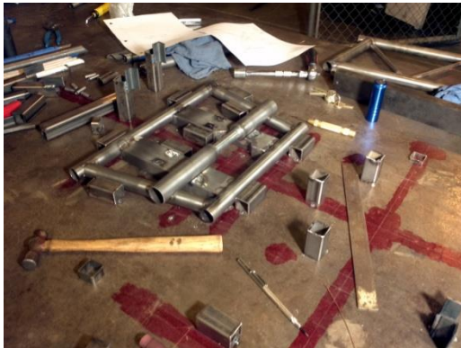
Figure 9.44 - Using a frame jig to make and weld the bulkhead together.
