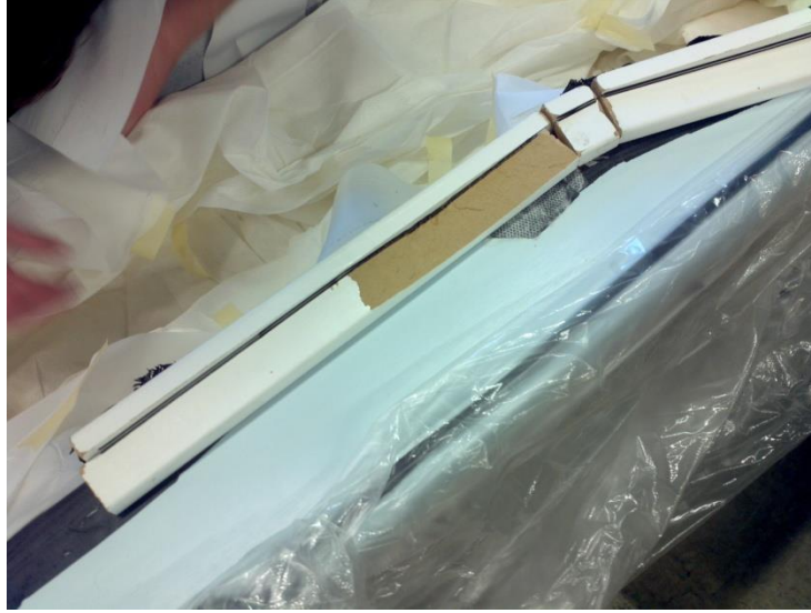
Figure 9.24 - The edge dams that had to be installed to prevent the core from being crushed under vacuum.
