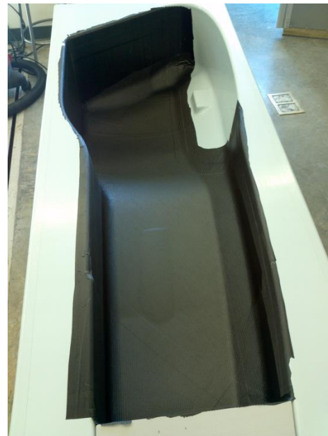
Figure 9.18 - The completed outer skin after an overnight debulk.
