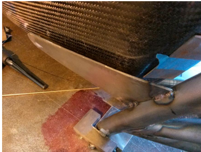
Figure 9.50 - Making the attachment plates to mount the monocoque to the rear frame.
