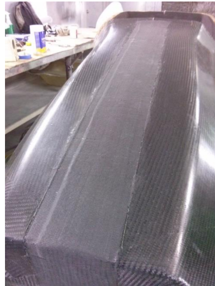
Figure 9.33 - The completed top lap joint.
