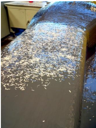
Figure 9.5 - Resin, plaster and chopped fiberglass applied to the buck.
