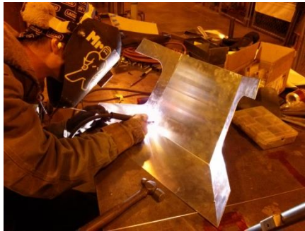
Figure 9.74 - Welding the head rest mount.
