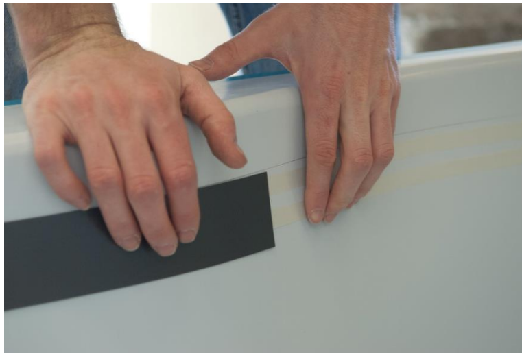
Figure 9.13 - Using high temperature double sided stick tape to place the two inch wide nylon strap for the lap joint step into the molds.
