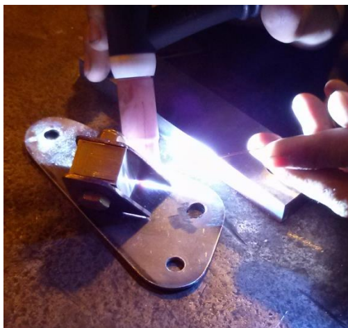
Figure 9.68 - Lap belt mounting tabs being welded in place.
