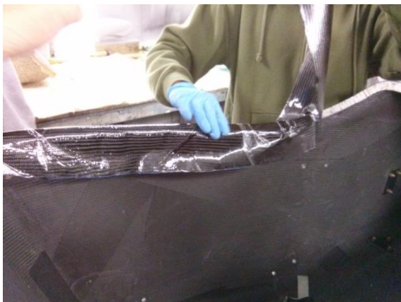
Figure 9.36 - Making the cockpit opening closeouts.
