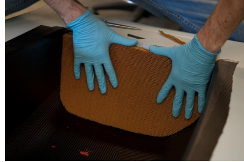
Figure 9.16 - Installing the front bulkhead sub-assembly.
