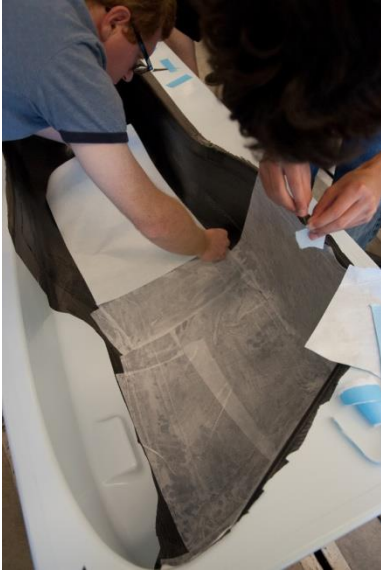
Figure 9.19 - Placing the film adhesive in the mold before the core goes in.
