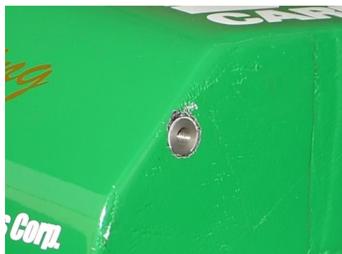
Figure 9.64 - Potted insert in front bulkhead.
