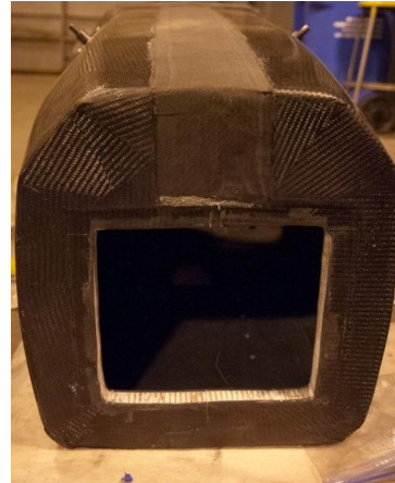
Figure 9.35 - Front bulkhead cut out after it was filled with microballoons.
