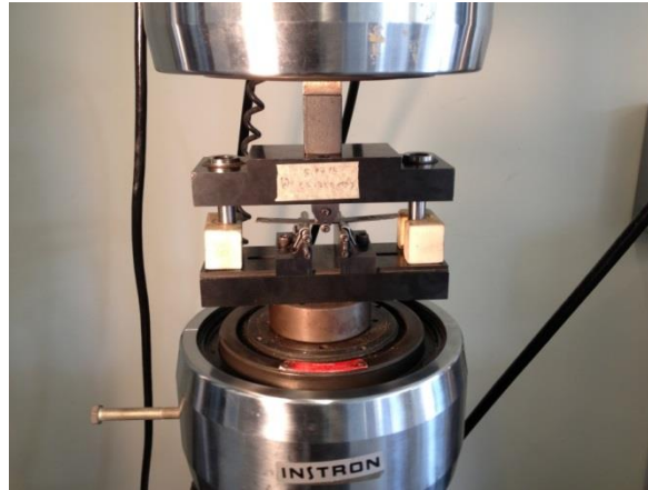
Figure 8.4 – ASTM 790 flex test setup.
