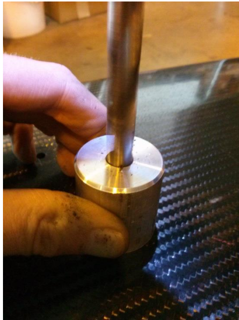
Figure 9.38 – Using a guide to drill a hole in the monocoque.
