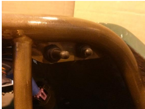
Figure 9.58 - Engine switches in place near the top of the front hoop.
