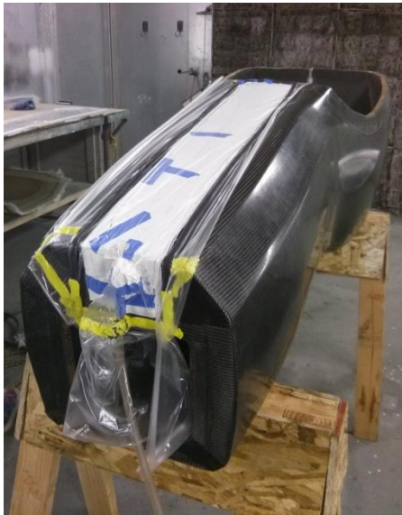
Figure 9.32 - The top lap joint lay up under vacuum.
