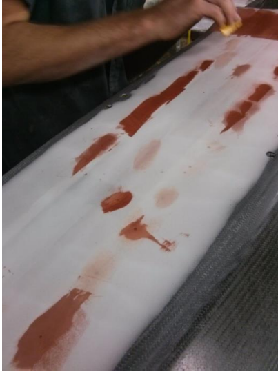
Figure 9.40 - The microballoon and resin surface (in white) and the glazing putty used to fill the pinholes.
