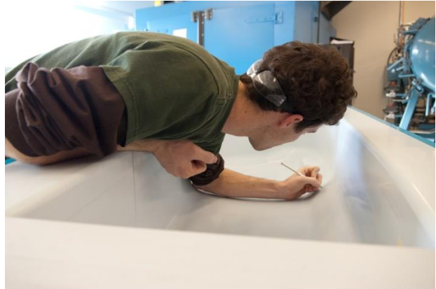
Figure 9.12 - Using a sharp scribe to clean out the scribe lines in the mold.
