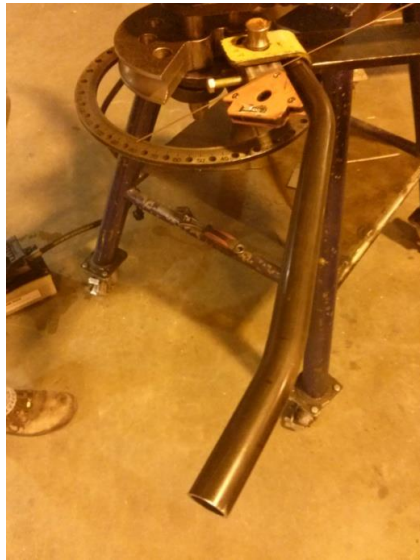
Figure 9.53 - Using the tubing bender to bend one half of the front roll hoop.
