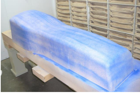
Figure 9.3 - A buck covered in guide coat and ready for sanding.
