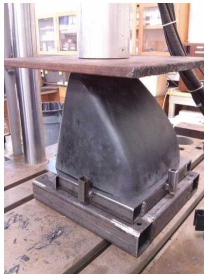
Figure 8.19 – Test setup for nosecone quasi-static crush test.
