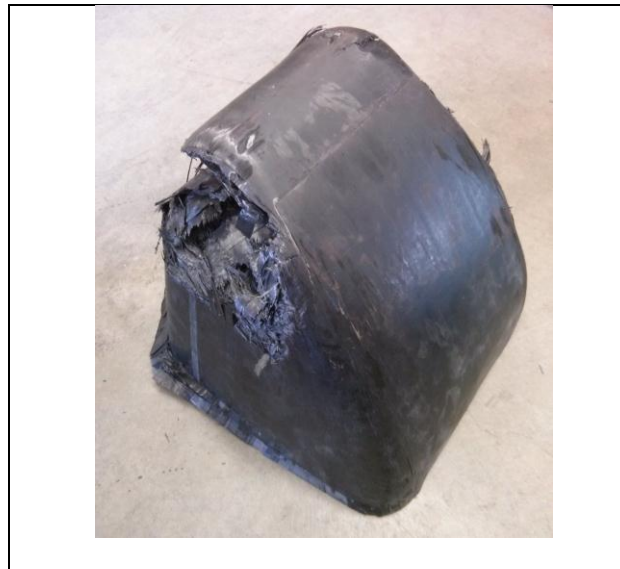
Figure 4: Attenuator after Impact (see attachment for AI plate)
