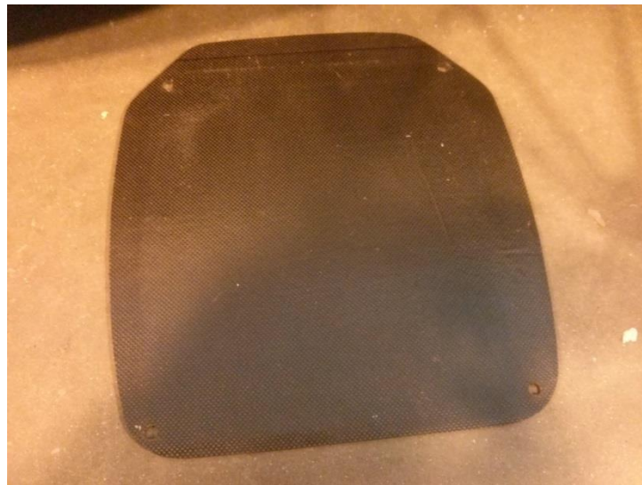
Figure 9.65 - The anti-intrusion plate ready to mount to the car.
