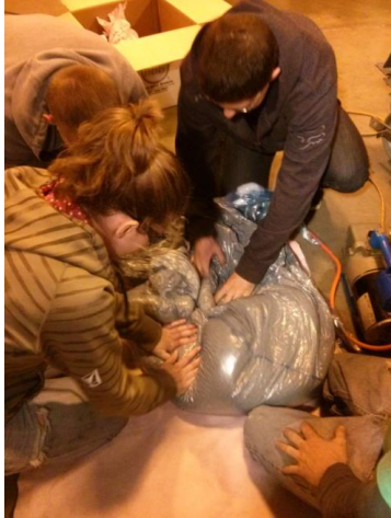
Figure 9.78 - Mixing the resin with the beads.
