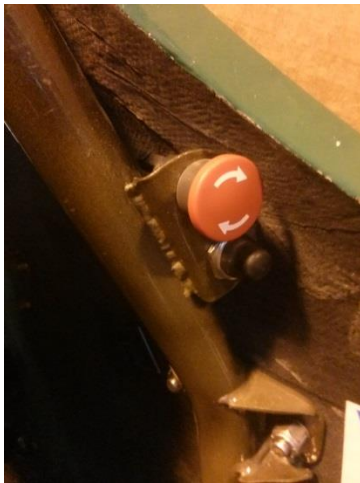
Figure 9.57 - The starter button and kill switch at the side of the front hoop.
