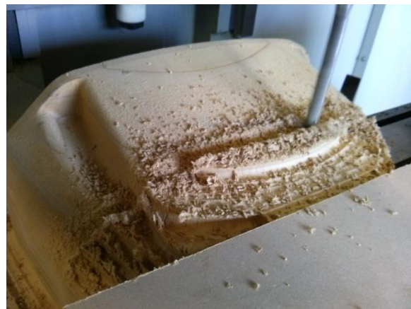
Figure 9.61 - The first operation in machining the nose cone buck.
