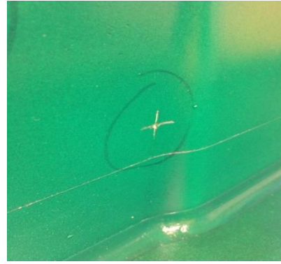
Figure 9.4 - The buck with the sealer applied and scribe lines scratched into the surface.
