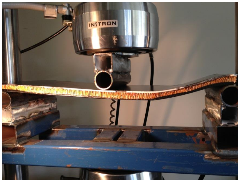
Figure 8.7 – Initial test piece “S” shape failure due to core shear
