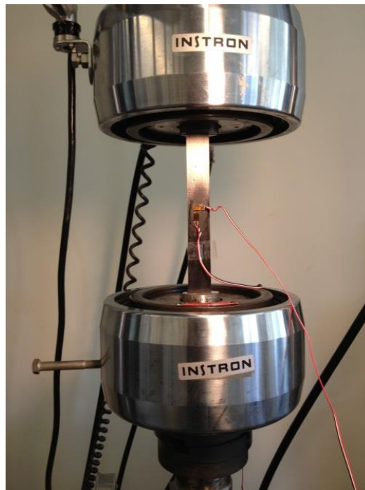
Figure 8.1 – ASTM 3518 45 degree tensile test set up.
