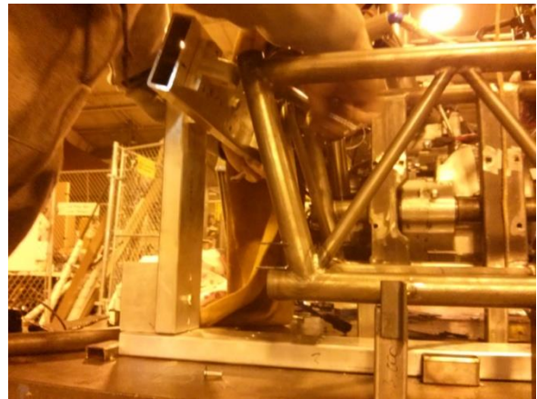
Figure 9.52 - Using the suspension jig to locate the rear suspension mounting tabs.
