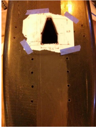
Figure 9.34 - The steering shaft cut out on the bottom of the tub.
