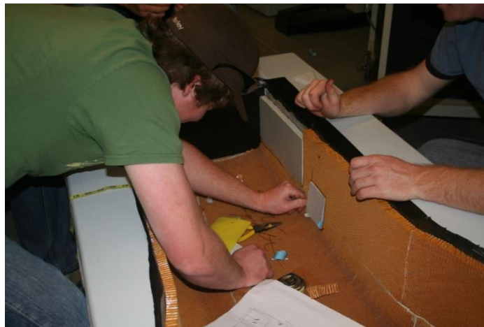
Figure 9.21 - Placing the end grain balsa inserts in for the lower front suspension mount and the pedal box.
