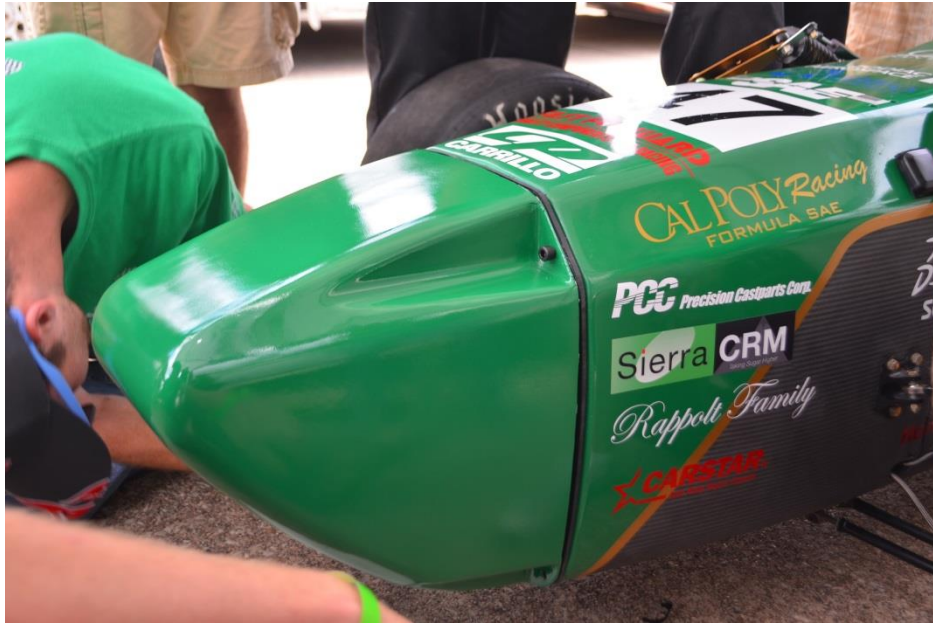
Figure 9.63 - Completed nosecone installed on the car. Anti-intrusion plate visible along base of the nosecone.
