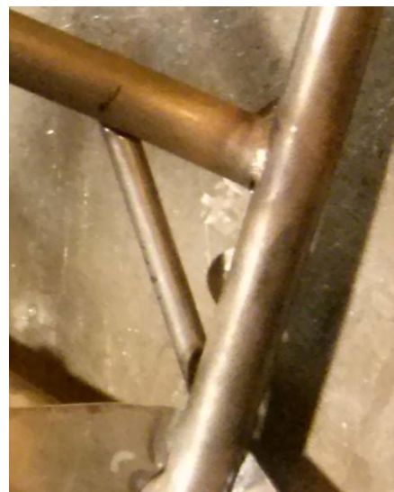
Figure 7.20 - Shoulder harness bar with gussets.
