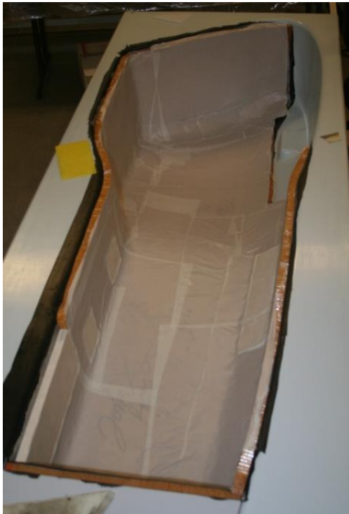
Figure 9.22 - The layer of film adhesive that was laid on the core in preparation for the inner skin.
