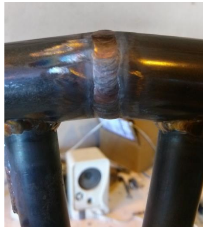
Figure 9.55 - The fully welded front roll hoop halves and steering mount.
