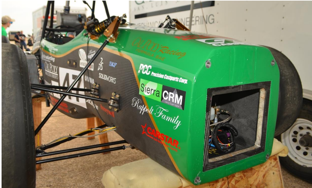
Figure 9.42 - The finished green paint and gold pinstripe. There is a satin finish on the exposed carbon and all of the sponsor stickers have been placed.
