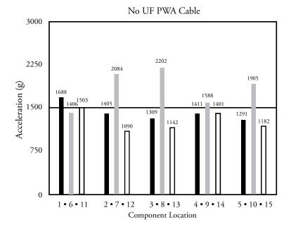
Figure 6. Accelerations on populated board with no cable and with cable.
