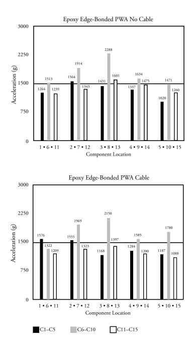
Figure 7. Accelerations on epoxy edge-bond populated board without cable and with cable.
