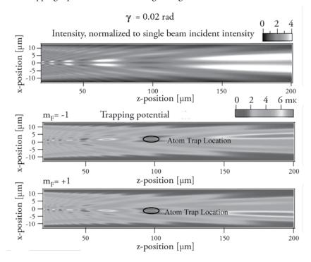
Figure 7. The intensity pattern and trapping potentials for a small angle ( $\gamma$ =0.02 radians) between the two lasers.
