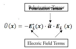
Figure 5. The compact form the light potential equation [6].
