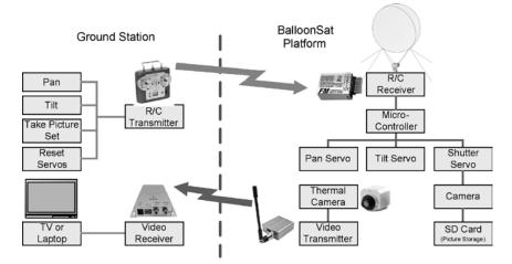
Figure 2. BalloonSat System Block Diagram
