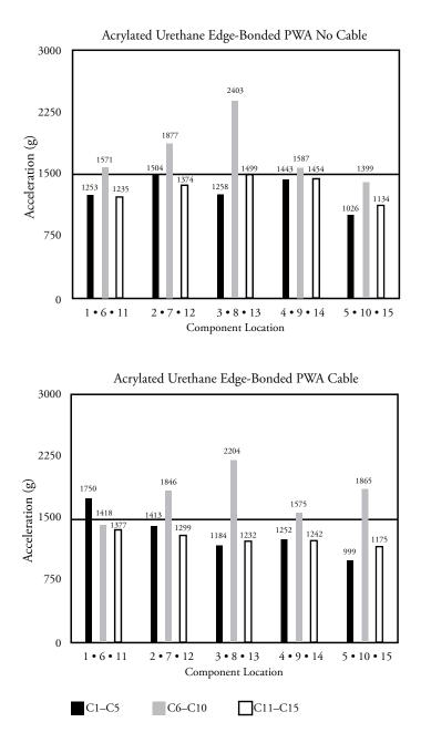
Figure 8. Accelerations on acrylic edge-bond populated board with no cable and with cable.
