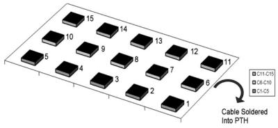
Figure 4. Cable in relation to component locations.
