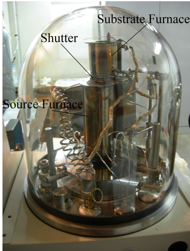
Figure 4.1: Hot Wall system of Epitaxy Laboratory, Physics Department of the Universidade Federal de Viçosa, Brazil. The legend in the figure shows two furnaces (substrate and source) that work independently and a shutter which allows starting/finishing the growth. The pressure during the growth can reach \sim 10^{-7} Torr.
