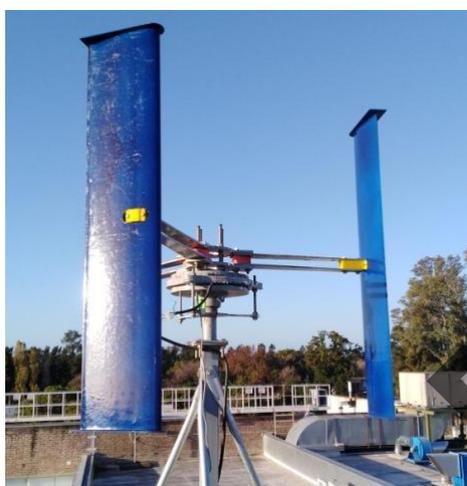
Fig 1. Aerogenerador Darrieus H.
