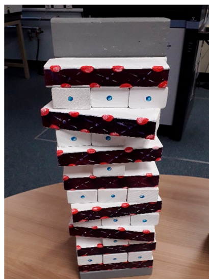
Figure 4. Oxide electrode tower block set showing that cobalt oxide layers have become displaced through the (de)intercalation of the lithium during cycle, thus showing degradation.
