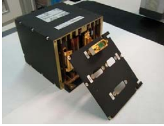
Figure 8. The electronic unit of the Langmuir Probe. (Thales Alenia Space).
