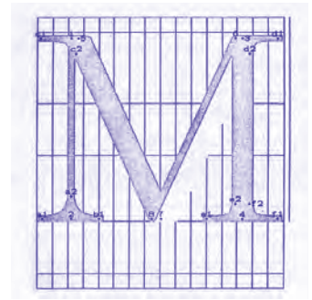
19 A proof of a Metafont constructed “M” (1981); different virtual pens drawing a stroke between the given coordinates.
