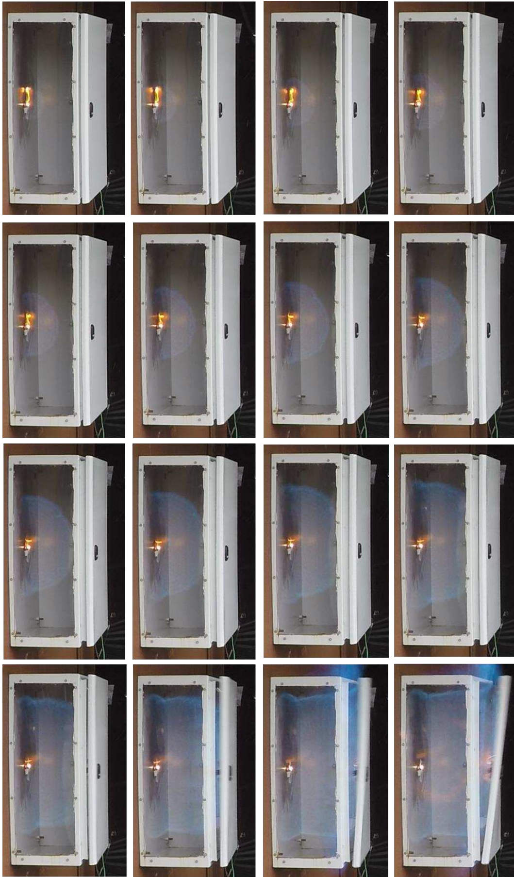
Figure 9 - Flame development in test 4; frame intervals 4.17 ms
