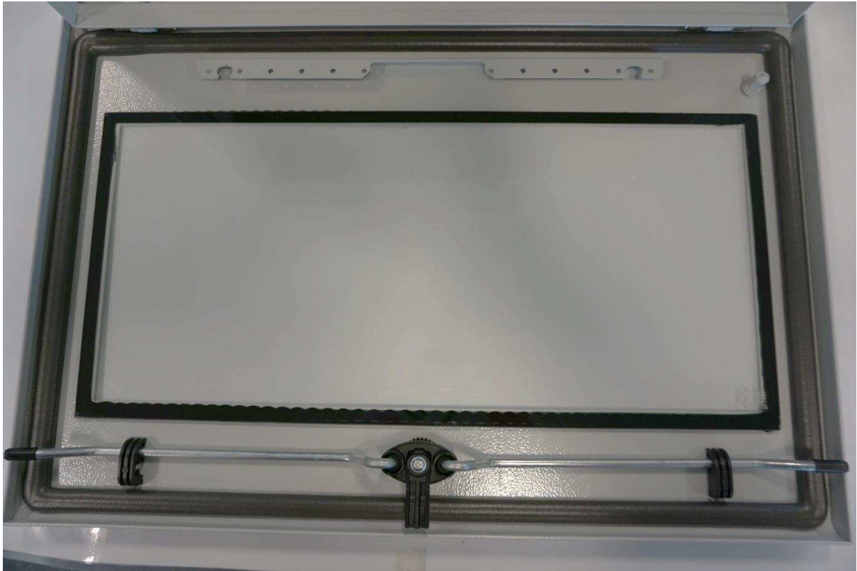
Figure 2- Three point locking mechanism of the control box doors
