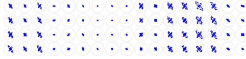
FIG. 3 (Colour online) Polar diagram of BiVO 4 under the polarization directions of polarizer and analyzer being parallel to each other. No SH signal is detected from the bulk region, and only the ferroelastic domain boundary exhibits SH-activity. The directions of SH maxima are the same for all domain boundaries that are parallel to the domain boundary.
