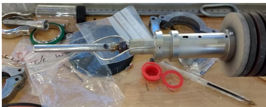
Figure 3.3. Filled vanadium can (containing alloy cylinders), attached to the sample holder with a thermocouple either side to monitor test temperature.
