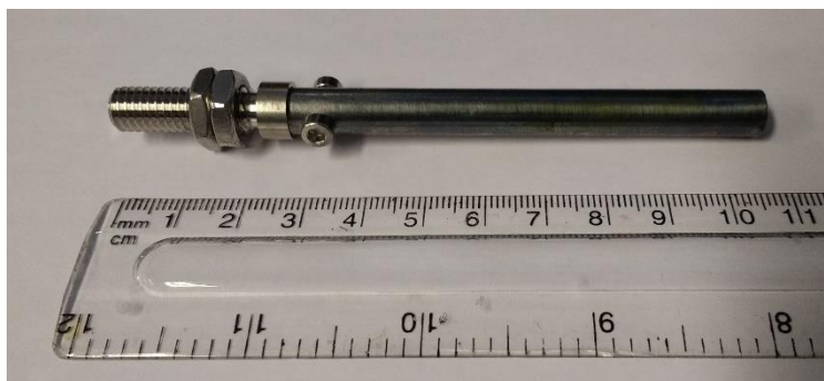
Figure 3.2. 8 mm diameter thin-walled vanadium can containing four aged alloy cylinders for one alloy composition prior to insertion into the sample holder.
