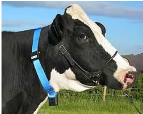
Figure 1. Silent Herdsman (Afimilk Ltd, Kibbutz, Afikim, Israel) 3-axis accelerometer based neck-mounted collar,
