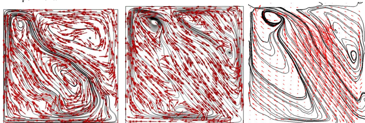
c) Case \theta=40^\circ , T_{\text{cold}}=60^\circ\text{C} , \Delta T=20^\circ\text{C} : Left - 2D simulation, Bi=0.526 , Ra=8.7 \times 10^7 , Ra_{\text{eff}}=2.66 \times 10^6 ; Center - 3D simulation, Bi=0.526 , Ra=8.7 \times 10^7 , Ra_{\text{eff}}=1.490 \times 10^5 ; Right - Experiment.
