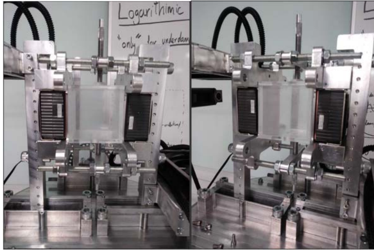
Figure 2: TCFS Test Rig with the 60 x 60 x 60 mm Perspex FC. Note that the Peltier Brackets, Peltier Devices and associated wiring have been removed for clarity:
