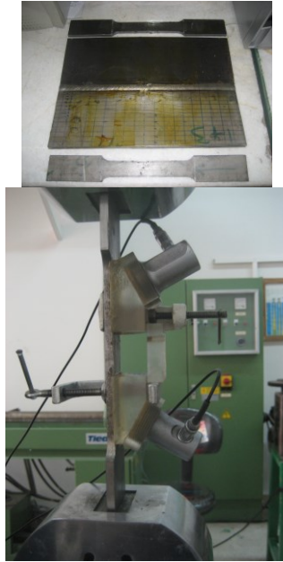
Fig. 8. Tensile test to evaluate acoustoelastic constant ( L_{11} ) in two different extracted samples
