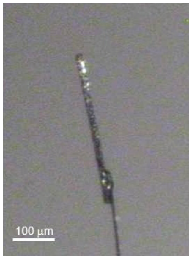
Figure 4. The single crystal of crookesite that was mounted for study on the XcaliburE four circle diffractometer, note the small size of this specimen.
