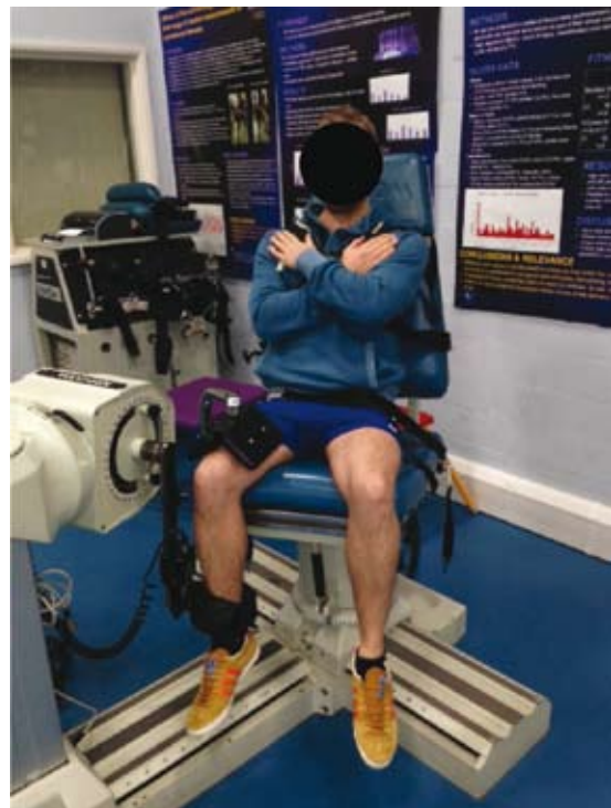
Fig. 1. Positioning of participant on the isokinetic dynamometer
