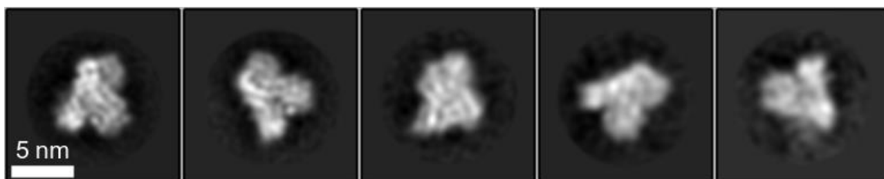
Figure 4.7. Best 2D classes generated from 3858 particles after data collection on a Talos Arctica 200 kV microscope. While promising secondary structure features are present, the limited variation in orientation of the classes hampered further data processing steps. The particles are only ~100 Å in length, ~20 Å shorter than the crystal structure.
