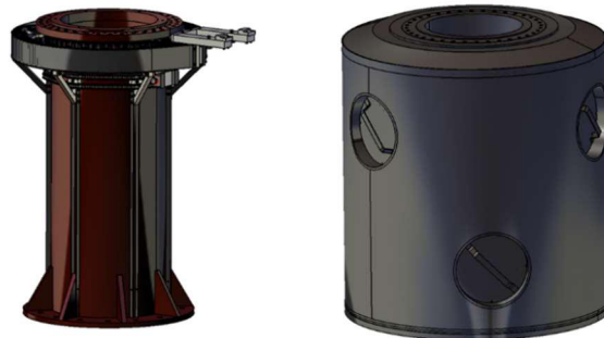
Figure 14. CAD views. On the left, pGCT tower with cable wrap. On the right, GCT pre-production tower design.
