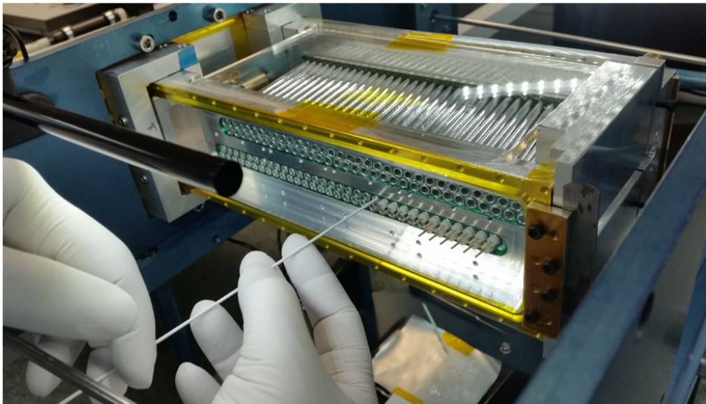
Figure 6.17: Photograph of a wire being threaded into a straw on the stringing jig.
