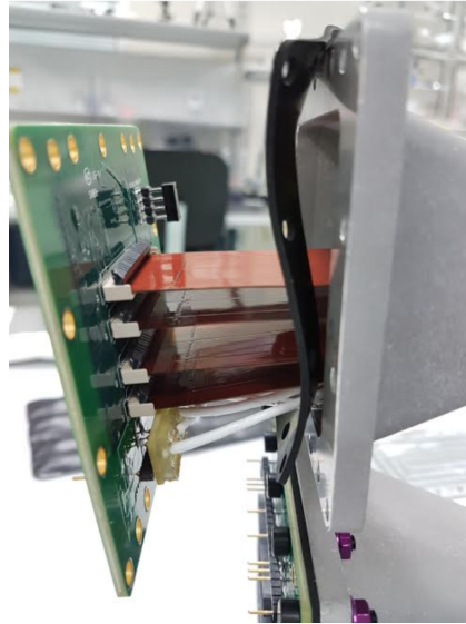
Figure 6.19: Photograph of flexi cables and HV internal cables connected to the feedthrough board.
