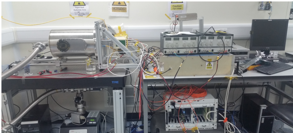
Figure 6.20: Clean room setup for module testing including the vacuum tank on the left and CAEN power supply on the right.
