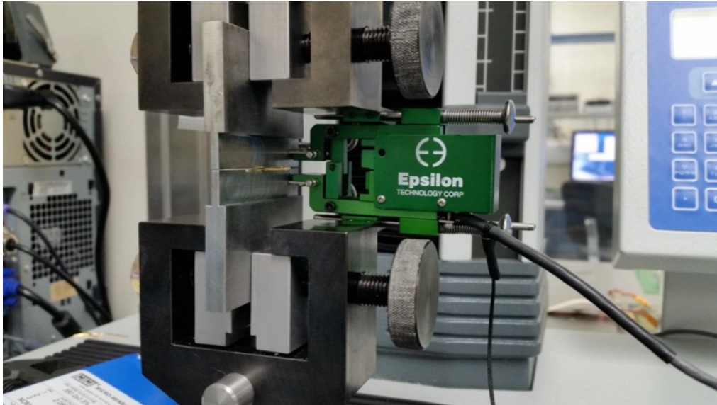
Figure 6.14: Photograph of the Lloyd LRXPlus materials tester crimping a pin.
