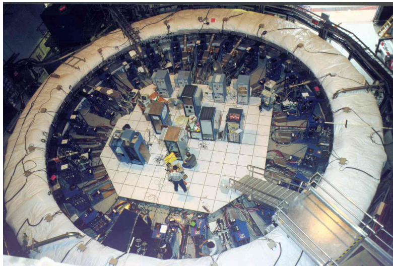
Figure 3.5: The storage ring of the BNL E821 experiment [2].
