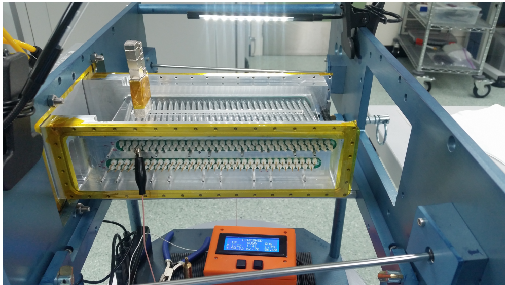
Figure 6.18: Photograph of a tension test being carried out on a wire.
