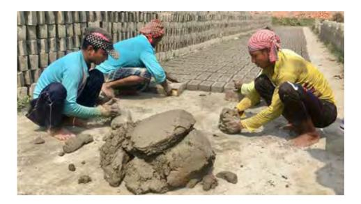
Brick-fields churn relentlessly in the dry season. Bricks are made by hand, sun-dried, fired and then cooled. Balls of tempered clay are thrown forcibly into wooden moulds before being skilfully turned out onto sanded, levelled ground. Moulding is repeated through rhythmic replications producing endless rows of unfired, green bricks are left to dry in the sun until they are firm enough to be fired, the drying dependent on circulations of the atmosphere
