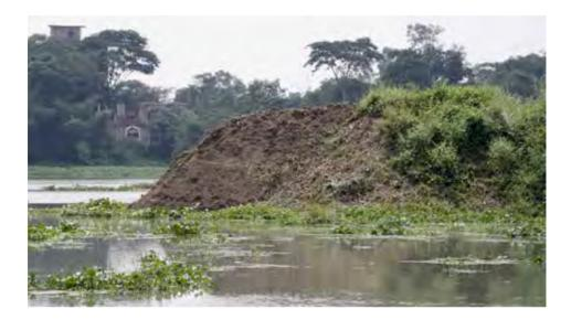
Clay soils are collected during the wet season in preparation for the dry season. Open-air stockpiles sit throughout the monsoon months, exposed to the action of the atmosphere. Rainwater spreads through the body of clay, diffusing and softening it. The action of wind, rain and air make it pliable for moulding, reducing human labour. Once the rains draw to a close, the water levels slowly start to recede, exposing the brick fields and allowing the brickmaking cycle to begin again.
