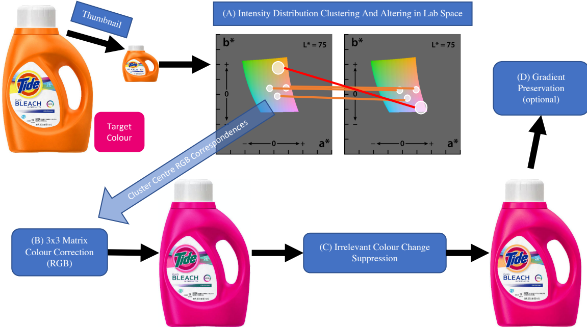
Figure 1: Primary colour editing pipeline. Given an input image, our method amends the product’s primary colour according to a target colour in 3-4 steps: A) Colour intensities clusters in CIE L^*a^*b^* colour space [29] are computed (left: original distributions; right: primary colour altered distributions); B) Cluster RGB correspondences are used for estimating a colour correction matrix. Note that the L^* channel intensities are also used for clustering but are not illustrated on the exemplar graphs; C) An alpha-blending process is applied to remove colour changes, which are less relevant to the primary colour change, from the colour corrected image; D) Some residual colour artefacts can be optionally removed using a gradient preservation method ‘regrain’ [26] (see the latter section for visualisation). The a^*b^* chromaticity gamut images are taken from Wikipedia [2].
