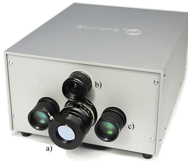
Fig. 1. Photo of the gas imaging camera. a) Lens of the SWIR FPA detector with attached filter. b) Lens for the colour webcam. c) lens tubes containing the two active illumination modules with visible engineered diffusers.
