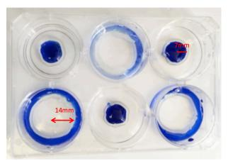
b. Second attempt at defining centre vs edge of wells. A 20ml syringe was used to syringe circles of petroleum jelly (Vaseline) onto the wells, using a laminated template placed under each well as an outline. 350µl RNA lysis buffer with a few drops of ink was carefully added to the centre or edge of the wells as before. No spillage occurred, and it was possible to scrape the wells without spillage too. Initial outlines were rough, but these improved with practice.
