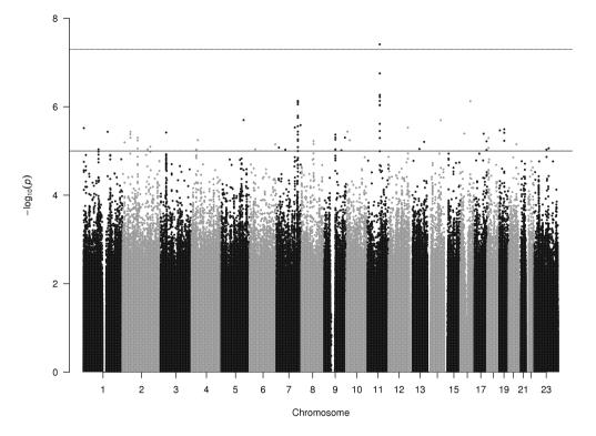
The y axis displays  $-\log_{10} p$  values of association -i.e. the "higher" the point on the graph, the more significant the association. The x axis is the position on each chromosome. Each dot represents a single SNP; however, these often overlie one another. The horizontal threshold lines represent a "suggestive significance" level threshold of  $p = 1x10^{-5}$  and a nominated genome-wide significance level of  $p=5x10^{-8}$ .
