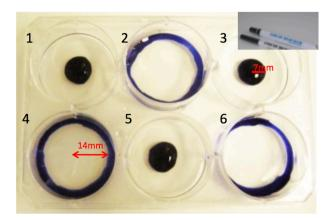
a. First attempt at defining centre vs edge of wells in a standard 6-well plate. A PAP pen (pictured in insert) was used to draw a hydrophilic boundary after shear exposure at diameters defined by fluid dynamics modelling (7mm or 14mm from centre). 350µl RNA lysis buffer with a few drops of ink was carefully added to the centre or edge of the wells. No spillage occurred initially, but on scraping the well to mimic extraction of RNA, spillage did occur.
