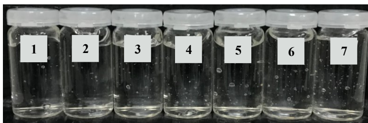
Figure 2.26. Images of the 0.15 wt% CU30 samples, containing mass fractions of NaCl ranging from 0.00- 3.13 \times 10^{-3} wt%. More specifically, the mass fraction of NaCl in the samples were: ‘1’ = 0.00 wt%, ‘2’ = 0.63 \times 10^{-3} wt%, ‘3’ = 1.25 \times 10^{-3} wt%, ‘4’ = 1.63 \times 10^{-3} wt%, ‘5’ = 2.13 \times 10^{-3} wt%, ‘6’ = 2.50 \times 10^{-3} wt% and ‘7’ = 3.13 \times 10^{-3} wt%. The pH values of each fluid were approximately constant, with pH values ranging from 7.23-7.54.
