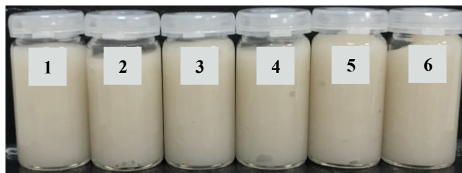
Figure 2.34. Images of the 6.00 wt% hectorite/CMC mixtures, ranging in CMC mass fraction from 0.525-3.75 wt%. More specifically, the mass fraction of CMC in the samples were: ‘1’ = 0.525 wt%, ‘2’ = 0.875 wt%, ‘3’ = 1.30 wt%, ‘4’ = 1.75 wt%, ‘5’ = 2.63 wt% and ‘6’ = 3.75 wt%.
