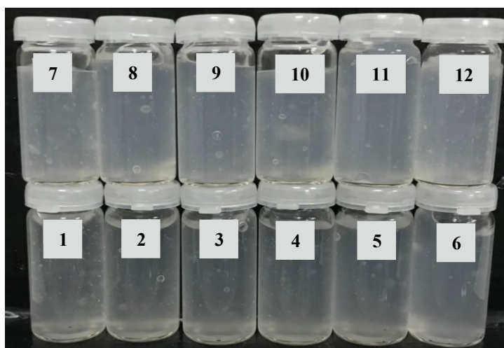
Figure 2.22. Images of the CU30 samples, ranging in mass fraction from 1.25-4.00 wt%. More specifically: ‘1’ = 1.25 wt%, ‘2’ = 1.50 wt%, ‘3’ = 1.75 wt%, ‘4’ = 2.00 wt%, ‘5’ = 2.25 wt%, ‘6’ = 2.50 wt%, ‘7’ = 2.75 wt%, ‘8’ = 3.00 wt%, ‘9’ = 3.25 wt%, ‘10’ = 3.50 wt%, ‘11’ = 3.75 wt%, ‘12’ = 4.00 wt%.
