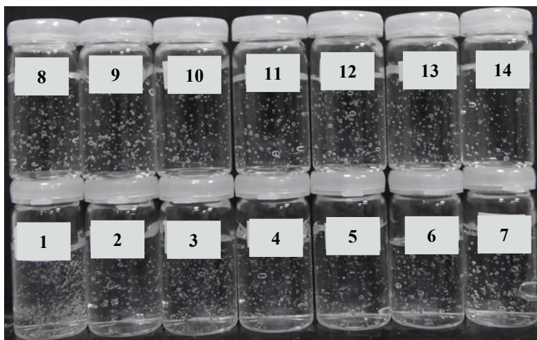
Figure 2.28. Images of the 0.80 wt% C981 samples, ranging in pH from 2.72-13.44. More specifically: ‘1’ = pH 2.72, ‘2’ = pH 3.52, ‘3’ = pH 4.07, ‘4’ = pH 4.76, ‘5’ = pH 5.23, ‘6’ = pH 5.74, ‘7’ = pH 6.22, ‘8’ = pH 6.64, ‘9’ = pH 7.30, ‘10’ = pH 8.49, ‘11’ = pH 8.78, ‘12’ = pH 11.66, ‘13’ = pH 12.83 and ‘14’ = pH 13.44.
