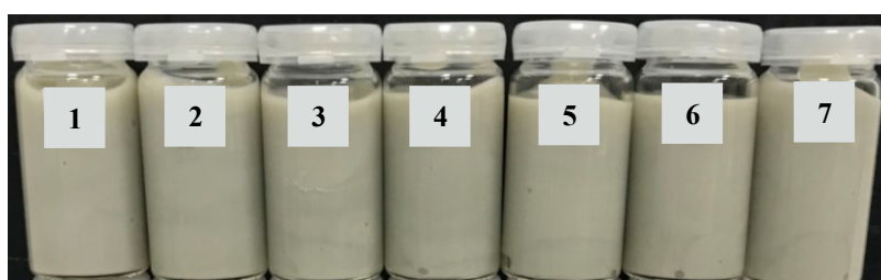
Figure 2.36. Images of the 14.91 wt% Actigel/CMC mixtures, ranging in CMC mass fraction from 0.700-2.18 wt%. More specifically, the mass fraction of CMC in the samples were: ‘1’ = 0.700 wt%, ‘2’ = 0.875 wt%, ‘3’ = 1.05 wt%, ‘4’ = 1.31 wt%, ‘5’ = 1.54 wt%, ‘6’ = 1.75 wt% and ‘7’ = 2.18 wt%.
