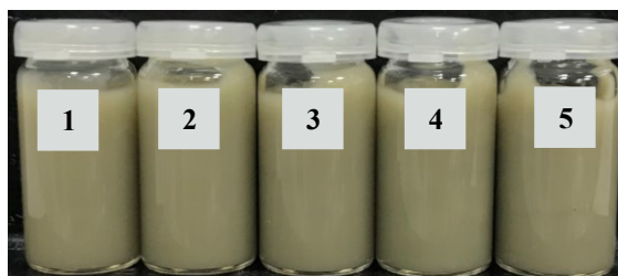
Figure 2.40. Images of the Bentopharm/glycerol mixtures, ranging in Bentopharm mass fraction from 8.50-10.00 wt% and glycerol mass fraction from 13.04-26.09 wt%. More specifically, the samples had the following mass fractions of (a) Bentopharm and (b) glycerol: ‘1’: (a) 8.50 wt%, (b) 26.09 wt%, ‘2’: (a) 9.00 wt%, (b) 21.74 wt%, ‘3’: (a) 9.50 wt%, (b) 17.39 wt%, ‘4’: (a) 9.75 wt%, (b) 15.23 wt% and ‘5’: (a) 10.00 wt%, (b) 13.04 wt%.
