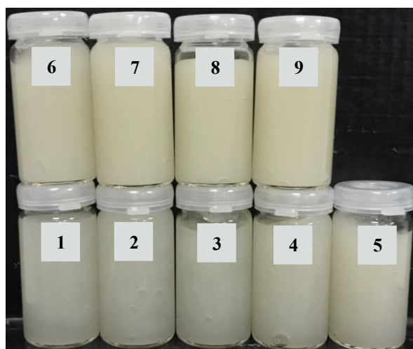
Figure 2.19. Images of the Actigum samples, ranging in mass fraction from 2.00-4.00 wt%. More specifically: '1' = 2.00 wt%, '2' = 2.25 wt%, '3' = 2.50 wt%, '4' = 2.75 wt%, '5' = 3.00 wt%, '6' = 3.25 wt%, '7' = 3.50 wt%, '8' = 3.75 wt% and '9' = 4.00 wt%.
