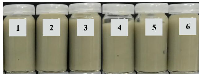
Figure 2.30. Images of the 8.50 wt% Bentopharm/CMC mixtures, ranging in CMC mass fraction from 0.175-1.83 wt%. More specifically, the mass fraction of CMC in the samples were: ‘1’ = 0.175 wt%, ‘2’ = 0.438 wt%, ‘3’ = 0.875 wt%, ‘4’ = 0.613 wt%, ‘5’ = 1.23 wt% and ‘6’ = 1.83 wt%.
