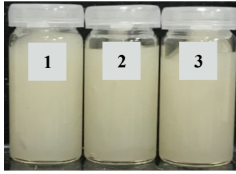
Figure 2.46. Images of 3.25 wt% Actigum/glycerol mixtures, with glycerol mass fraction ranging from 0.00-18.75 wt%. More specifically, the samples had the following mass fractions glycerol: ‘1’ = 0.00 wt%, ‘2’ = 12.50 wt% and ‘3’ = 18.75 wt%.
