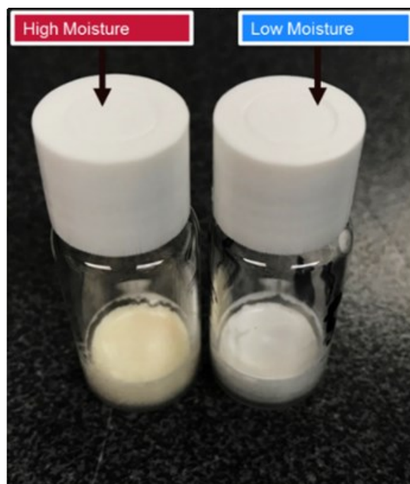
Figure 5.33 Comparison of the visual appearance between vials FD in either “low” or “high” moisture cycle for IgG 50 mg/mL after 12 months storage at 45°C.
