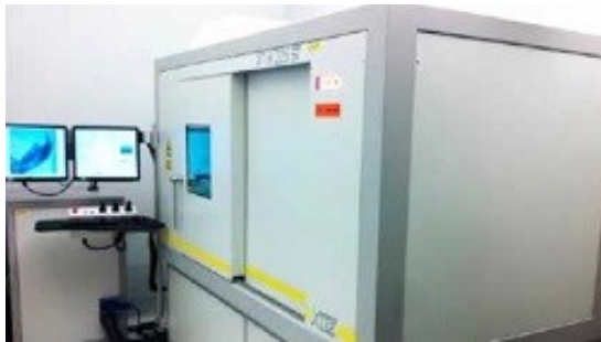
Figure 4-27 Metris X-Tek HMX ST 225 CT scanner in the Natural History Museum, London.
