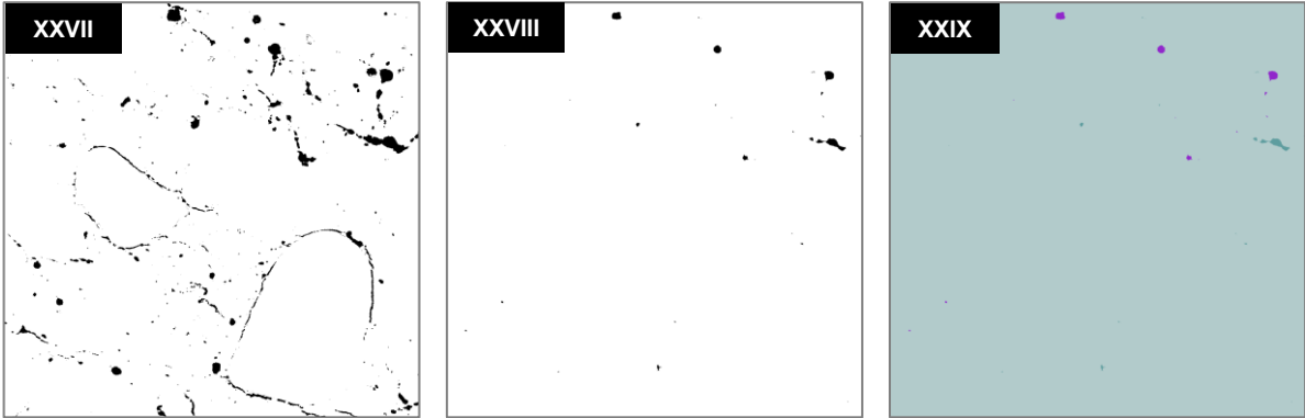
Figure 6-17 Image processing: XXVII) Result of subtraction: (Image XXIII) - (Image XXVI); XXVIII) Image after binary erosion using a ball as a structuring element with half-kernel size of 6; XXIX) Manual selection of remaining air voids.
