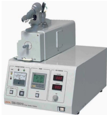
Figure 4-17 JEOL SM-09010 Ar-BIB cross-section polisher at RWTH Aachen University, Germany.
