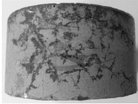
Figure 4-9 Microcrack pattern of concrete sample (C/SF-14/SC) subjected to autogenous shrinkage.
