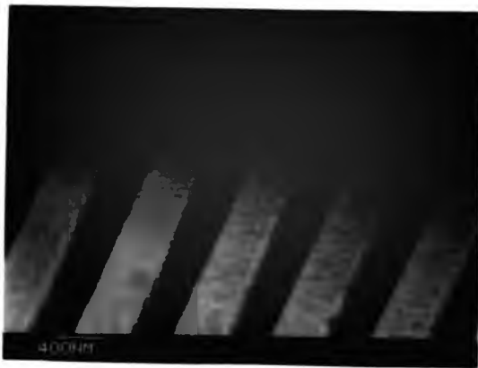
FIGURE 55 Nominal 250 nm 1:2 Lines and Spaces 10 mol % (MMI)-co-MMA. Exposure Dose 215 \mu\text{C}.\text{cm}^{-2} 8:2 n-Butyl Acetate : n-Hexyl Acetate Mix.
