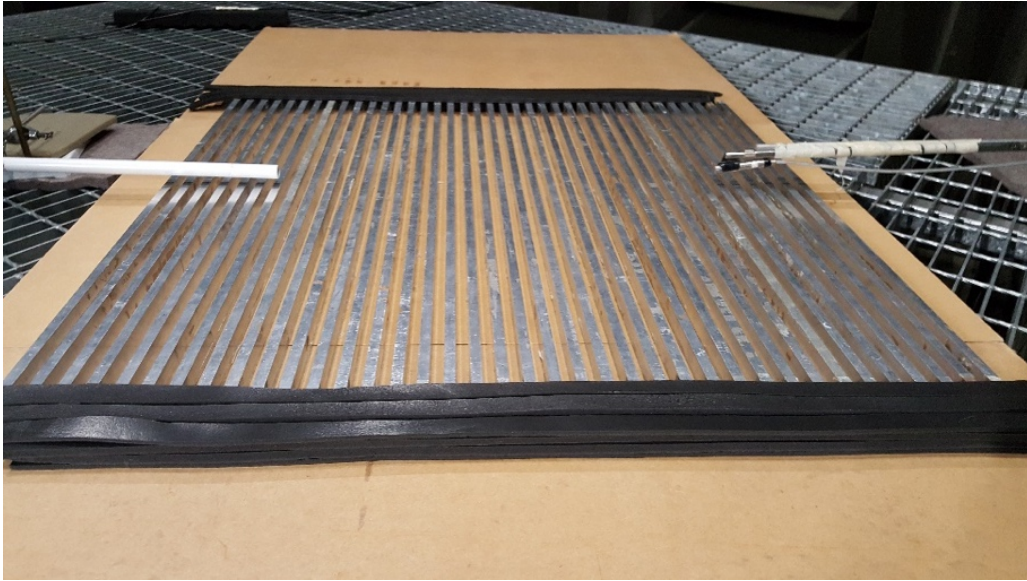
Figure 5. 11 Experimental setup for strips with felt placed at each end of the strip array.
