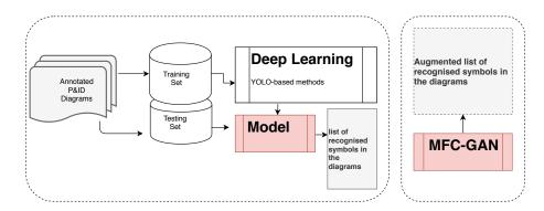
Figure 2: Schematic diagram of the framework for processing and analysing engineering documents
