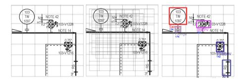
Figure 4: The method divides the P&ID Diagram into a grid, following the YOLO model [55], and predicts the class probabilities of the bounding boxes. The figure shows the symbols sensor, flange, DBBPV, DB&BBV and RS
