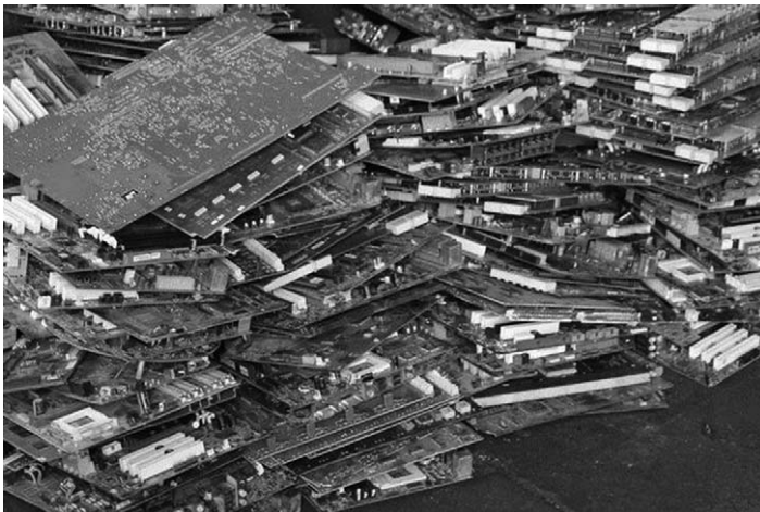
Figure 10.1 Bulk PCB WEEE containing mixed metals and components.
