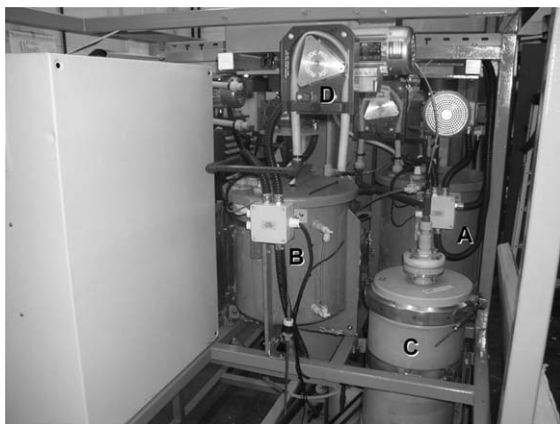
Figure 10.17 Pilot plant (50 L scale) for the operation of a DES-based process for Ni recovery and recycling from Ni plating waste generated by the surface finishing PCB supply chain and battery waste.
