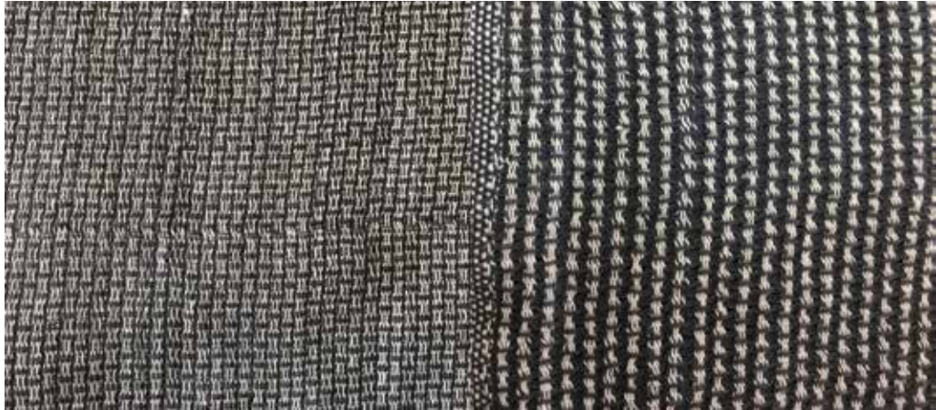
Figure 7.39: Sleeve Panel Before and After Finishing: Loom State (Left) and Finished (Right) (2018) Photograph by Anna Piper
