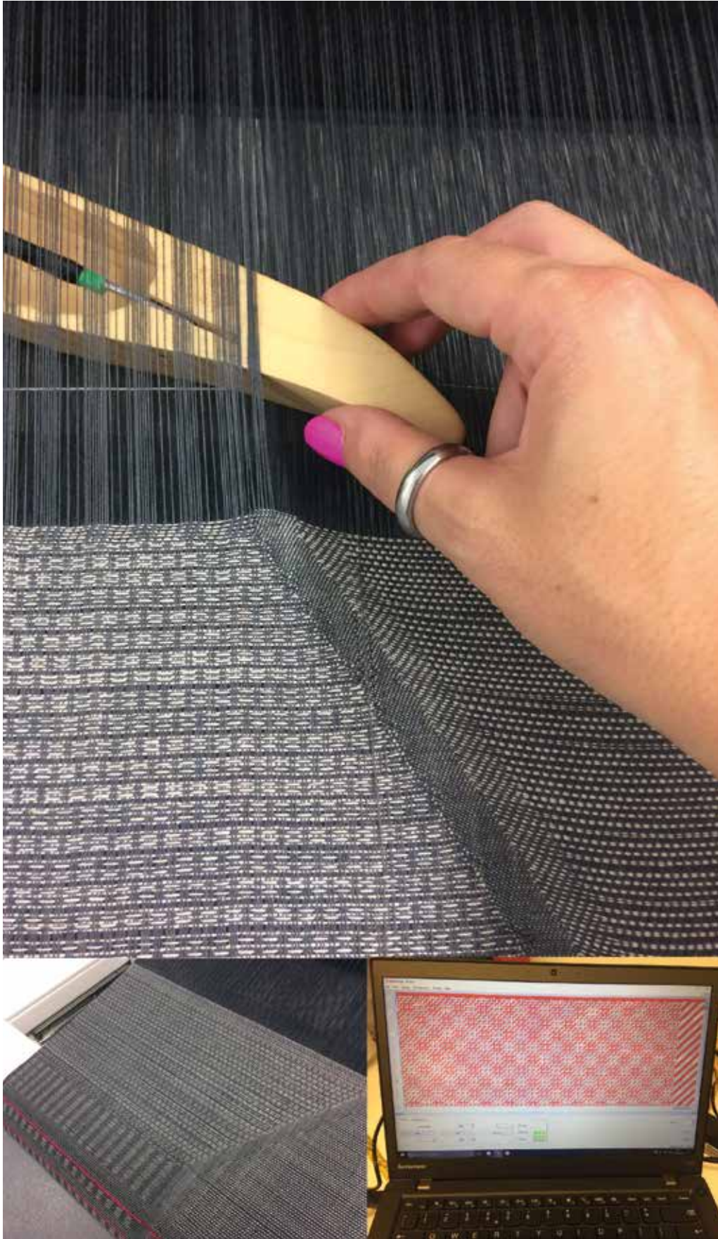
Figure 2.9: Garment Construction on the TC2 Loom Based on a Pre-programmed Design (2018) Photographs by Anna Piper
