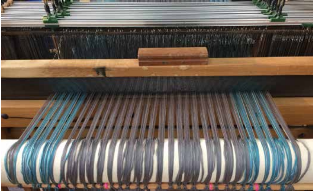
Figure 4.13: The Reed Determining the Width and Density of the Warp (2017)
