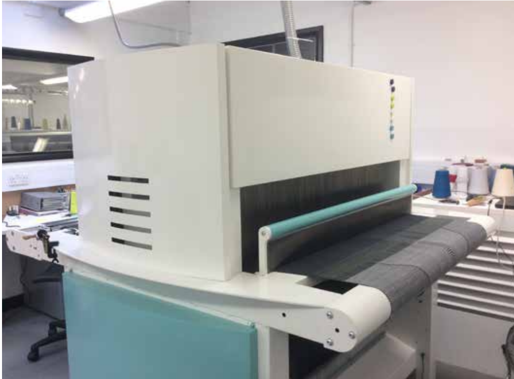
Figure 7.4: TC2 Jacquard Sample Loom with Modular Thread Controller (2018) Photograph by Anna Piper
