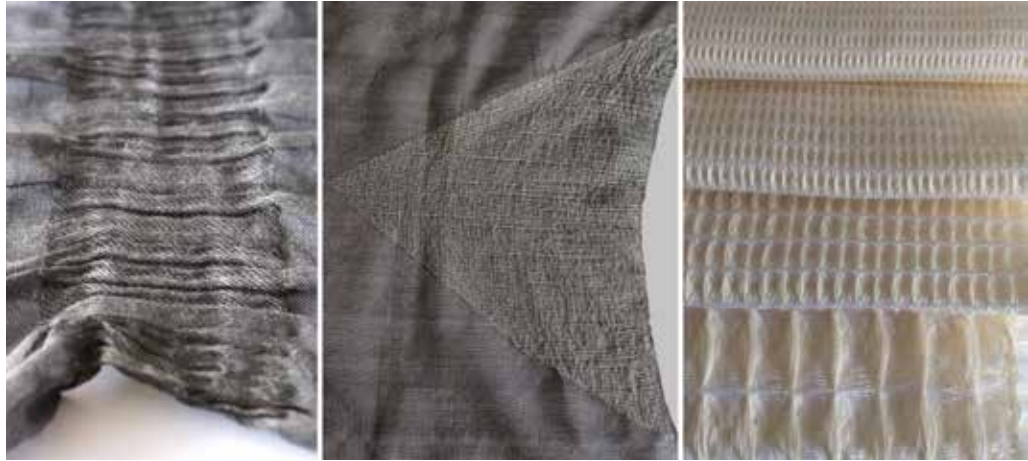
Figure 7.13: Fabric Types: Self-pleating, Panelling and Cellular Structures (2015) Photographs by Anna Piper
