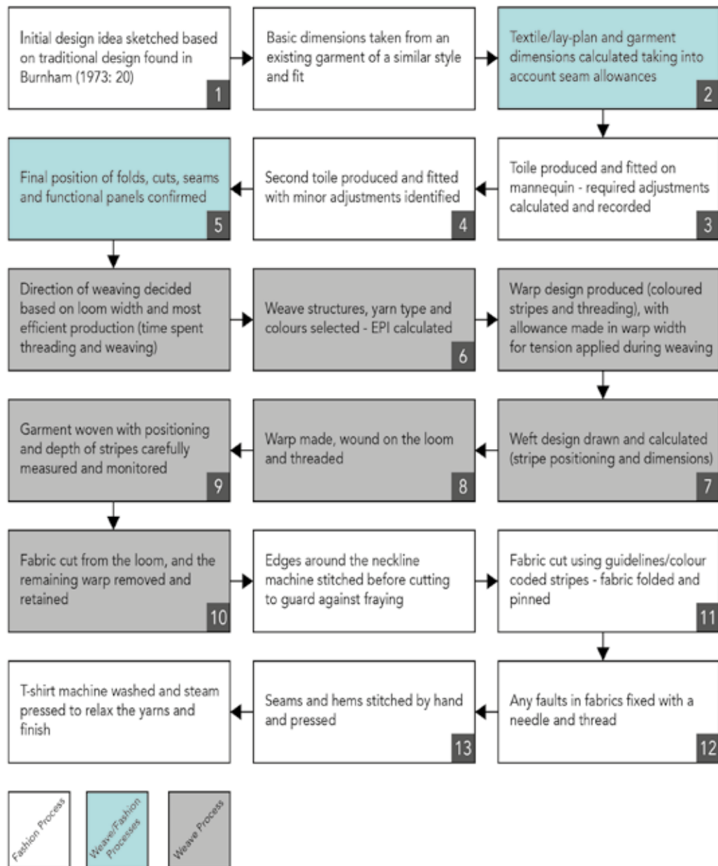
Figure 7.22: Hand Woven T-shirt Production Process (2018)
