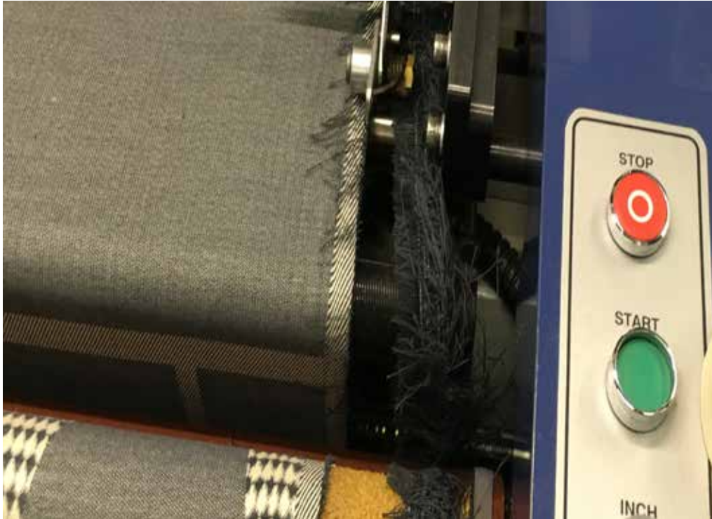
Figure 7.28: Jacquard Power Loom: Cutting Away of False Selvage (2018) Photograph by Anna Piper
