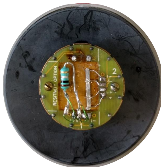
Figure 4.3 : Titanium alloy bar mounted on PPMS resistivity puck for transport measurements.
