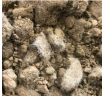
Figure 3.5 Fibre aggregation when fibres and soil were mixed using the wet mixing method.
