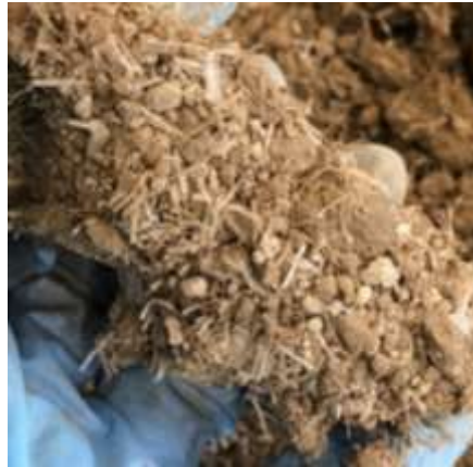
Figure 3.3. The accumulation of fibres in a fibrillated fibres-soil mixture (0.3% fibre inclusion ratio).
