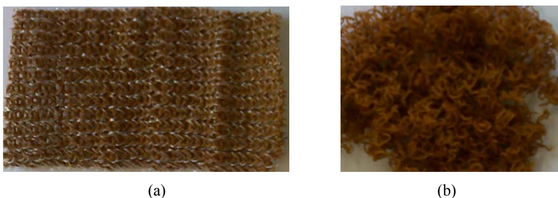
Figure 3.1. PAN fibre based catalyst: (a)-knitted mesh, (b)-catalytic threads
