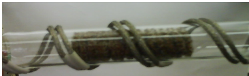
Figure 5.17. Packing of catalytic mesh (discs) in the dynamic reactor
