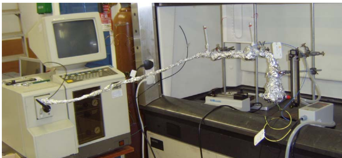
Figure 5.1. Dynamic experimental rig used for the oxidation of EtSH in dry conditions, wrapped in foil for better heat insulation
