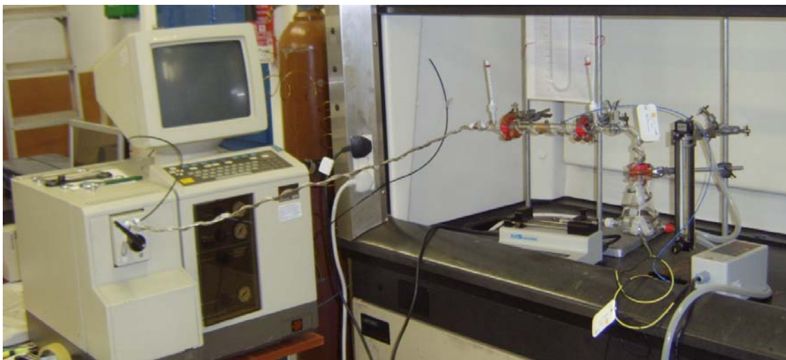
Figure 5.2. Dynamic experimental rig used for the oxidation of EtSH in dry conditions, with full view of the heating system
