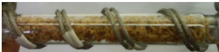
Figure 5.5. Packing of catalytic threads in the dynamic reactor
