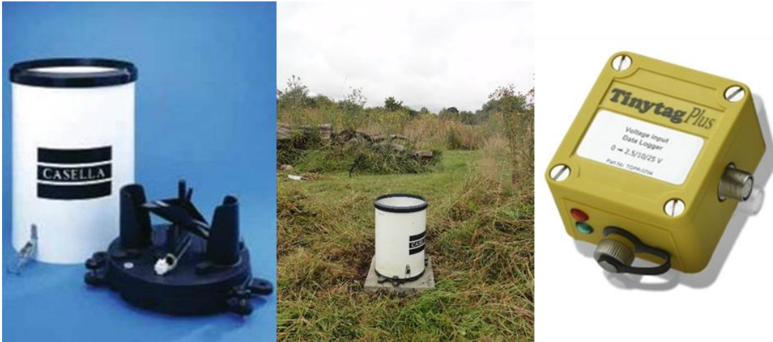
Figure 3.7: Precipitation measurement using a tipping bucket rain gauge (left) located in an open area (centre) with data collected using a reed logger (right) (photo of rain gauge courtesy of Casellasolutions.com, photo of reed logger courtesy of geminidataloggers.com)
