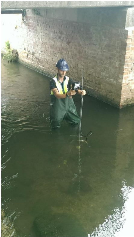
Figure 3.6: Spot gauging of flow using Flow-Tracker
