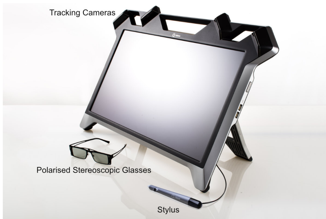
Figure 2.13 The immersive zSpace 200 display, featuring 6 degrees of freedom stylus, passive stereoscopic glasses, tracking cameras and 3D monitor (Source: zSpace, Inc [203]).
