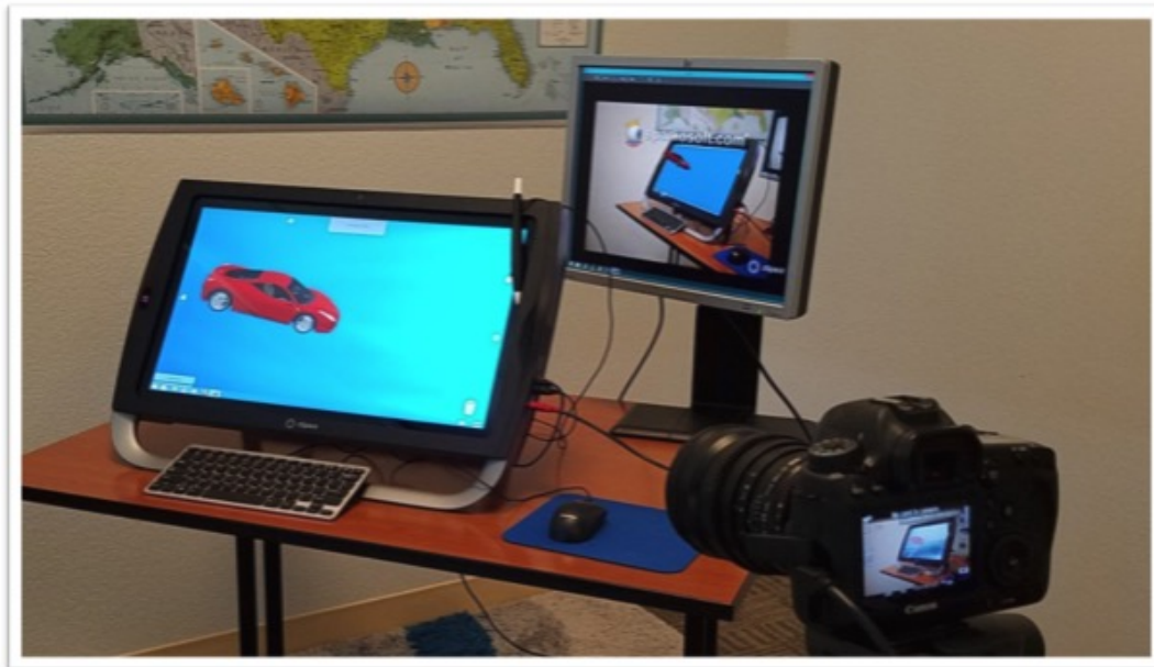
Figure 2.14 The zSpace zView collaborative view mode, achievable with a video camera and secondary screen. The secondary monitor renders the virtual objects as they would appear to the primary zSpace user while wearing the stereoscopic glasses (Source: zSpace, Inc [206]).
