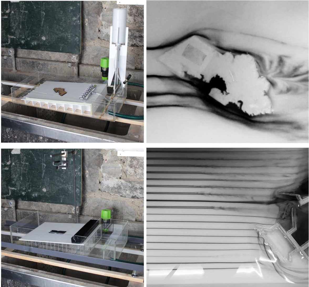
Figure 17. Water tables V2 and V3 were integrated with the sink, relying on gravity for drainage. Reduced surface spans and adjustable feet facilitate steady-state flow. Additional components aid in calibration. Images: Emma Bennett.
