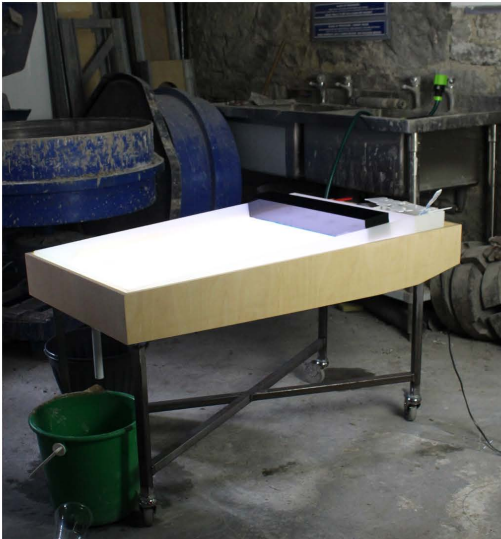
Figure 16. Water table V1 suffered from deflections and leaks, causing water to pool towards the center of the table. Images: Emma Bennett.
