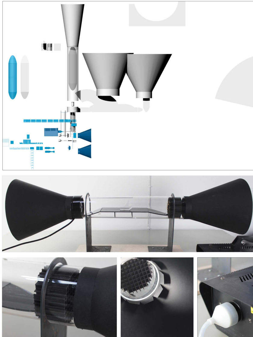
Figure 10. (top) Wind tunnel V2 was developed as a digital model. (middle) A cylindrical testing section and digitally fabricated elements facilitate smooth transitions between components. (bottom) The resultant model reconciles the need to create an interior environment minimizing turbulence with an exterior form of smooth transitions and tight tolerances. Drawing and Images: Author.
