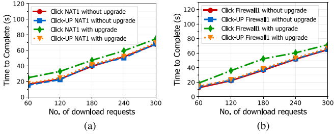
Fig. 13. Comparison of time taken to satisfy completed requests between Click-UP and native Click. (a) Click NAT1 and Click-UP NAT1. (b) Click Firewall1 and Click-UP firewall1.
