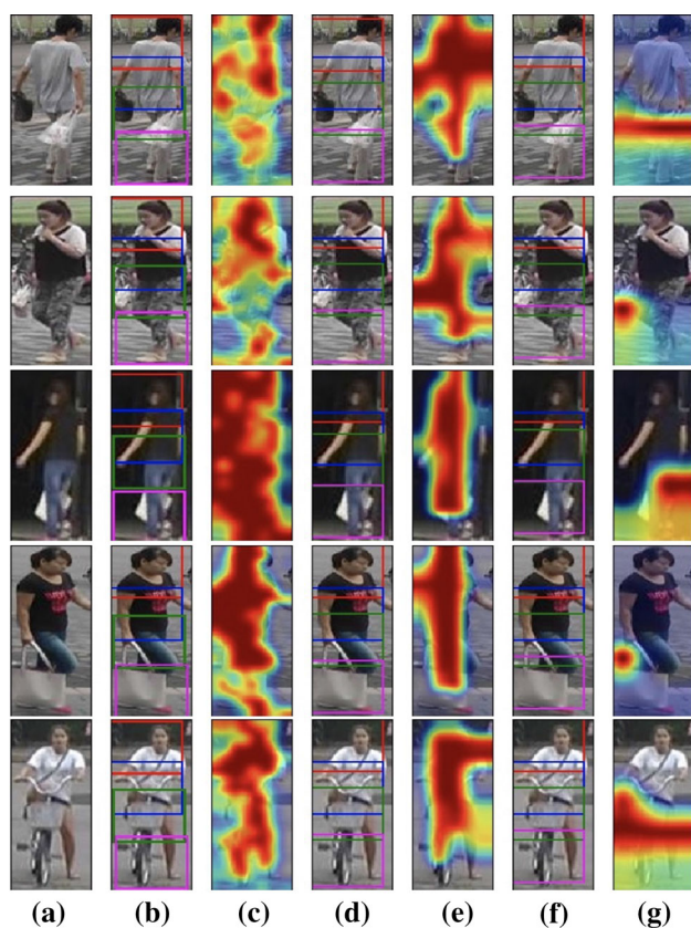
Fig. 7 Visualisation of the harmonious re-id attention. From left to right, a the original image, b the 1st-level of hard attention, c the 1st-level of soft attention, d the 2nd-level of hard attention, e the 2nd-level of soft attention, f the 3rd-level of hard attention, g the 3rd-level of soft attention
