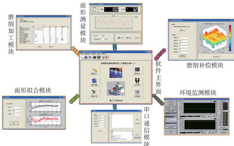
图5 计算机辅助制造软件功能模块关系图 Fig.5 Relationship of CAM functional sub-system
