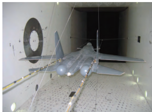
(b) 跨声速风洞悬浮支撑 [43]
