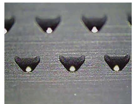
图3 气膜冷却异型孔结构 Fig.3 Shaped film-cooling hole configuration
